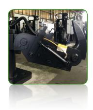
In the event of a breakdown or failure, it is possible to open the hooks on the unit manually. A demountable lever prevents accidental opening.
